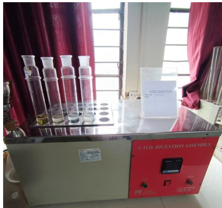
Figure 4 C.O. D. Testing Apparatus
