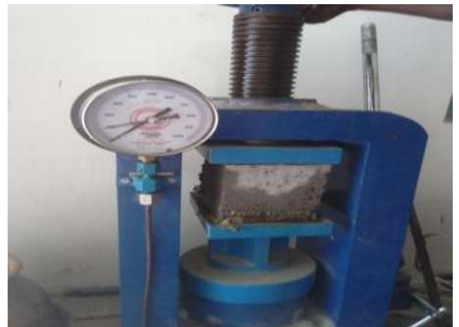
Fig- 5: Compression testing Machine
