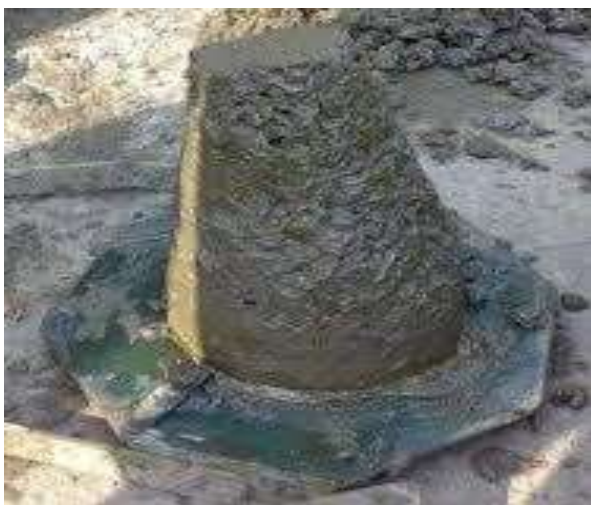
Fig -3: Sample of concrete mix for Slump Test
