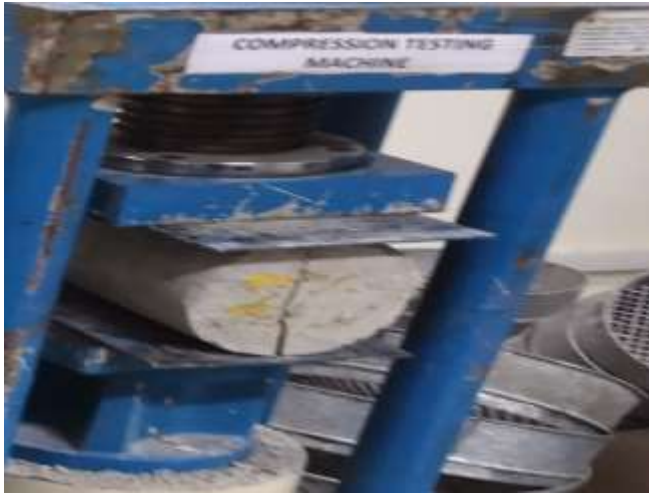
Fig 4.2: Crack pattern observed on cylinder specimen
