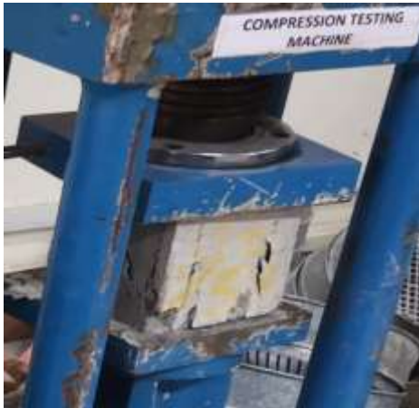
Fig 4.1: Crack pattern observed on cube specimen
