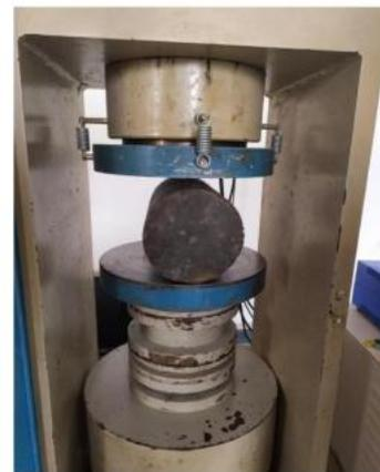
**Fig:** Universal testing machine
