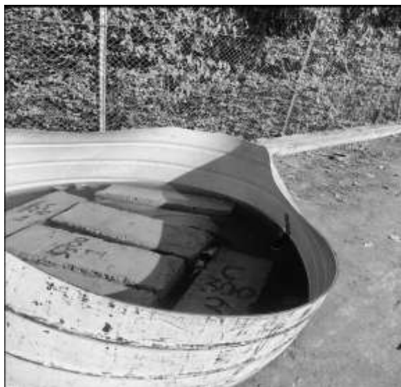
Fig. 2. Column specimens undergoing 28-day water curing
