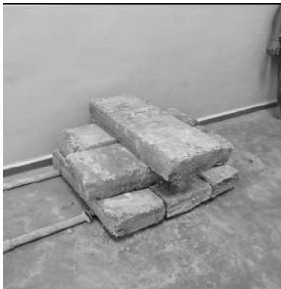
Fig. 3. Cured column specimens after 28-day curing, prior to axial compression testing
