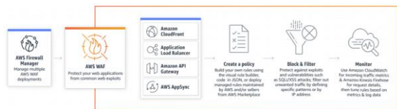
Figure 4: AWS WAF Security Automations uses AWS CloudFormation to block SQL injection attacks
