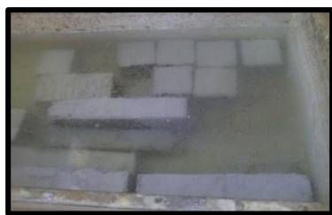
Fig: 3. Curing of Concrete Specimen
