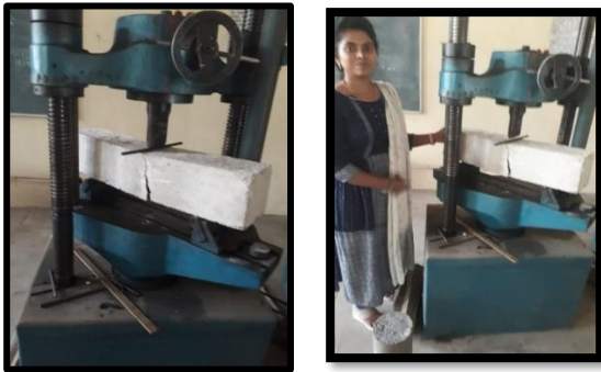
Fig: 6.2.3 Flexural Strength Test
