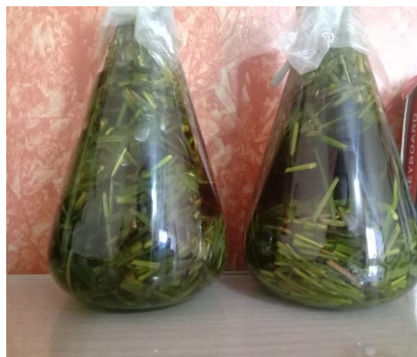
Fig. Extraction of Lemongrass substrate using Ethyl Acetate solvent
