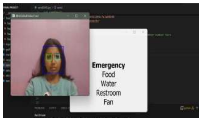
Fig. 3. Real-time eye-tracking system selecting the "Emergency" option to assist a Locked-In Syndrome patient in communicating basic needs.
