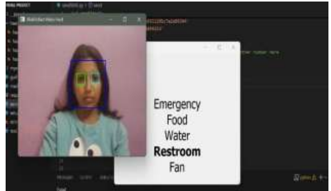
Fig. 4. Real-time eye-tracking system selecting the "Restroom" option to assist a Locked-In Syndrome patient in communicating basic needs.
