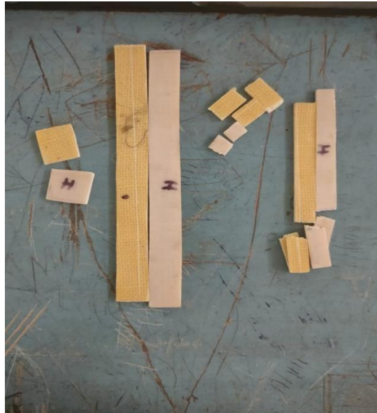
Figure 3.6 Hybridization of bamboo with pineapple fibre reinforced with Epoxy composite
