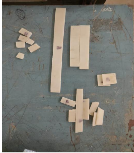
Figure 3.4 Bamboo fibre reinforced with epoxy composite
