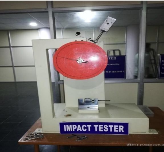
Figure 3.10 Impact machine for impact testing Impact strength was calculated by the following relation
