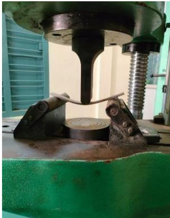
Figure 5.4: Flexural Testing Machine
