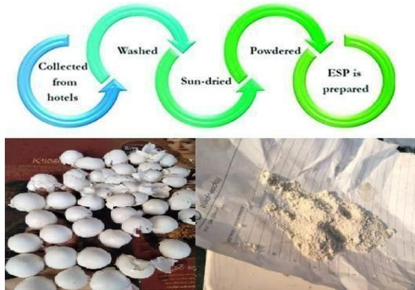
Figure 3.5: Duck Egg Shell Powder Processing
