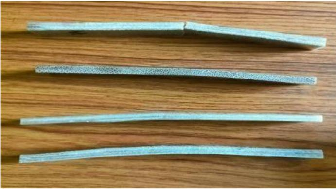
**Figure 5.5: Flexural Test Specimens After Testing**
