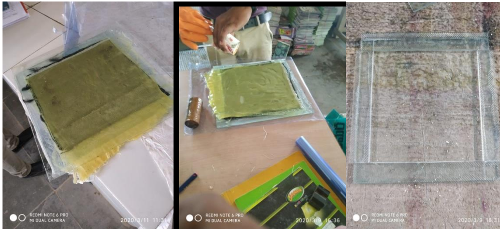
Fig: Hand Lay Experimental Set up
