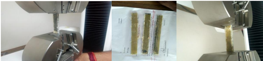
Fig: 3.9: Tensile Specimens and testing (150x15x3mm)
