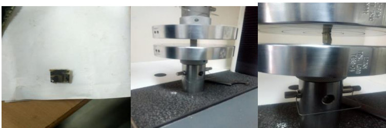
Fig: compression test specimen and testing
