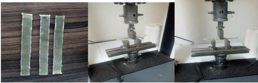
Fig: flexural test specimen and testing
