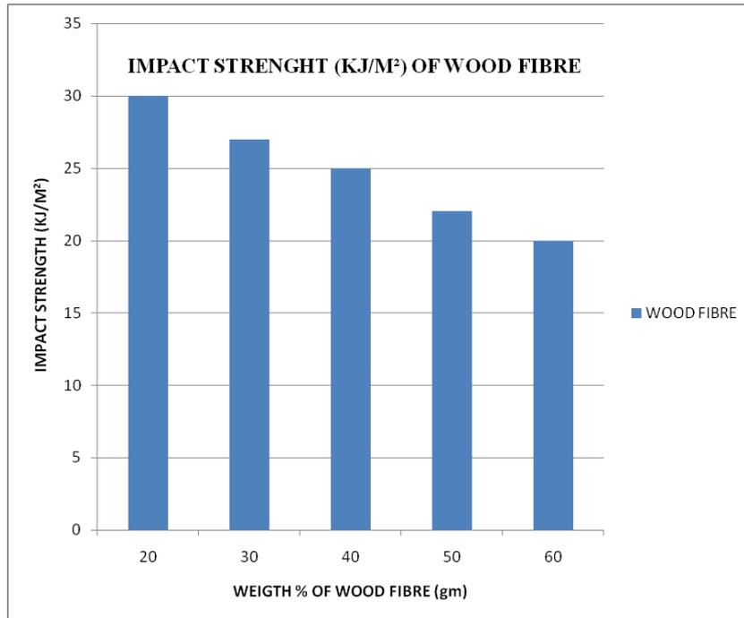
The Impact Testing test was conducted on Charpy Pendulum Impact Testing Machine the Impact load is applied on the specimen 20,30,40,50,60 Respectively and the impact strength is achieved 30,27,25,22,20 (KJ/M<sup>2</sup>).
