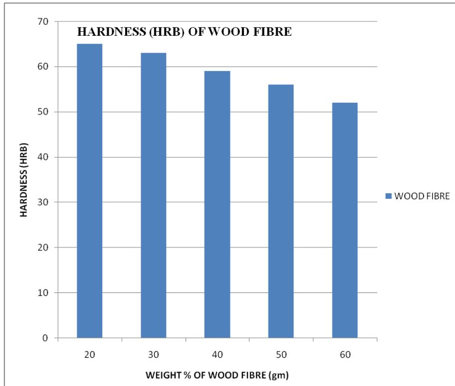
The hardness test was conducted on Brinell Hardness Machine. 20,30,40,50,60 are the weight percentage of the wood fiber. The hardness achieved in the test is 65,63,59,56,62 Respectively
