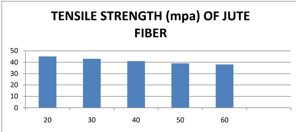
On testing on Universal Testing Machine The tensile strength was achieve as per 20 gm of jute fiber and 250gm of Polypropylene (PP) we get Maximum Permissible Stress is 45mpa similarly on 30gm,40gm,50gm,60gm we get Maximum Permissible stress(mpa) is 49,46,44,42 and 40 respectively
