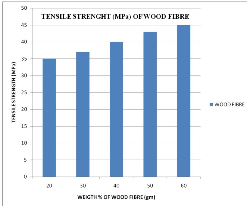
similarly on wood fiber Tensile strength The Maximum Permissible stress (mpa) is 34,35,41,42,44 on Flax fiber weight ratio that is 20,30,40,50,60(gm) Respectively.
