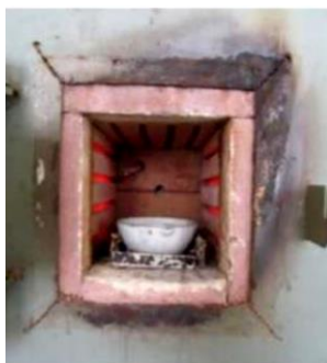
Fig 2: Heating the pellets at 590°C
