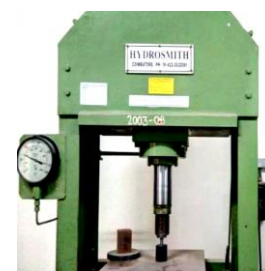
Fig 6: Compaction using Hydraulic press
