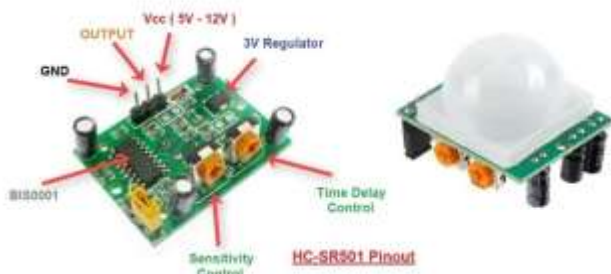
Figure 5. HC-SR501 PIR Sensor
