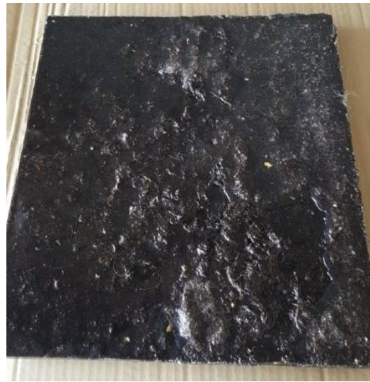
Figure 7: Rough surface on the bottom part of the top plate due to excess excess amount of hardener.
