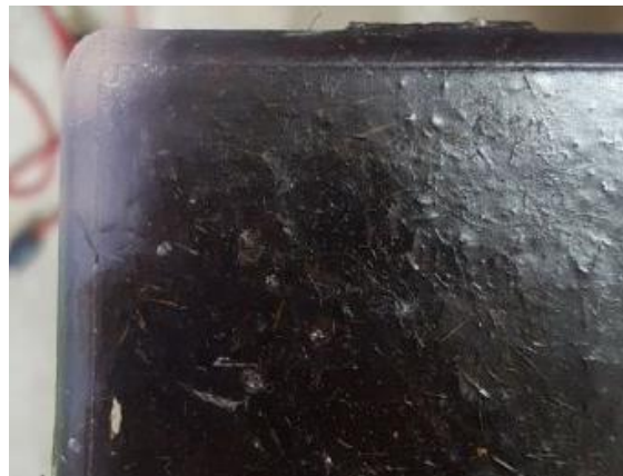
Figure 8: Failure in compressing the fibre in mould.
