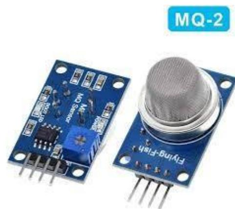
The sensor works on the principle of change in conductivity of the sensing material present in it. This material is exposed to the surrounding air and when a target gas comes in contact with it, there is a change in its conductivity. This change in conductivity is then
