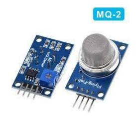
The sensor works on the principle of change in conductivity of the sensing material present in it. This material is exposed to the surrounding air and when a target gas comes in contact with it, there is a change in its conductivity. This change in conductivity is then
