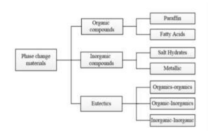
**Fig. Classification of Phase Change Material**
