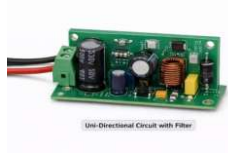
Figure 4.5 Uni-Directional Circuit with Filter
