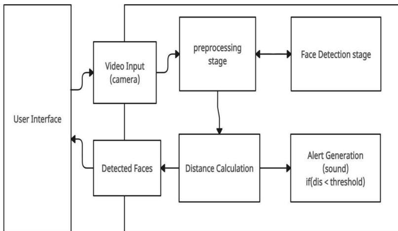
Figure 4. System Architecture.
