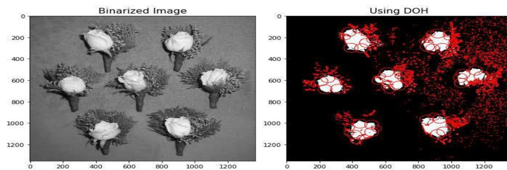
Figure 2. Feature Detection and Matching with blobs.
