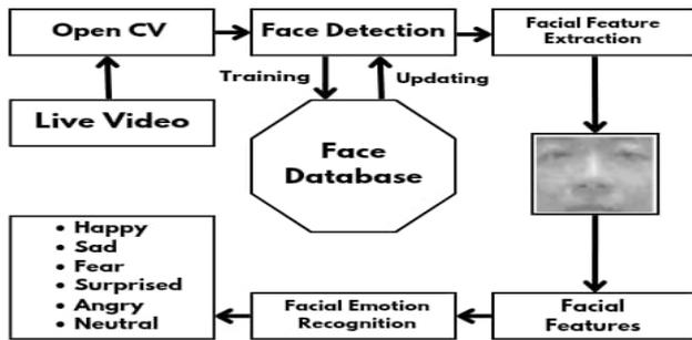
Fig.1 Architectural design for Proposed work
