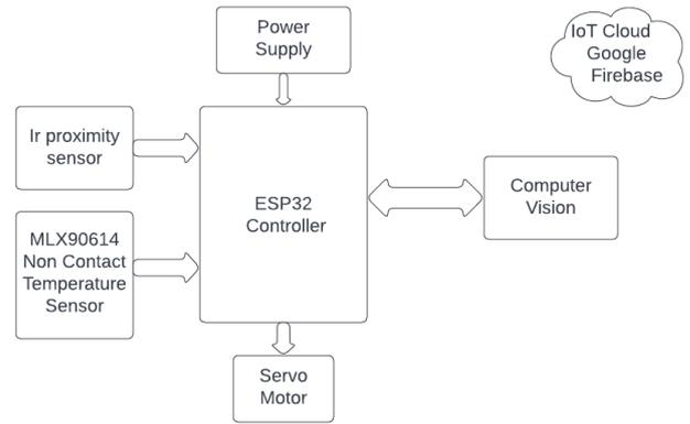
Fig -2: Block Diagram of Face Mask Detection
