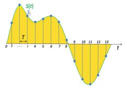
Fig: Signal sampling representation
