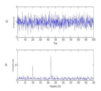
The time series and (b) frequency spectrum of a signal
