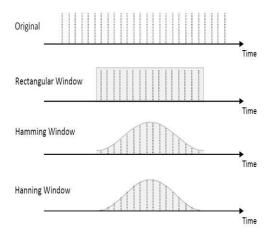
Fig The effects of different window functions on a digital signal
