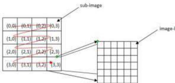
Fig. Definition of Sub-image and Image-block in the EHD
