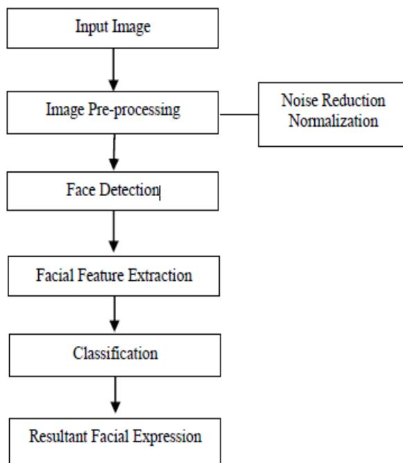
Fig: Facial emotion recognition block diagram
