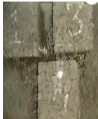
Curing of cube Specimen in ambient conditions
