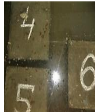
Curing of cube Specimen in ambient conditions
