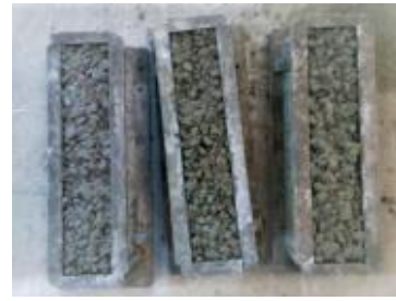
finishing of top surface of concrete in cube and beam
