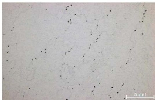
Figure 15. Oriented creep cavities in nose cone support weld
