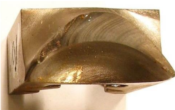
High cycle fatigue failure of steam turbine airfoil.
