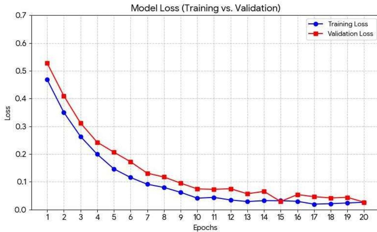
The loss curve demonstrates a smooth exponential decay. Both training and validation loss follow a nearly identical downward path, which is the primary indicator of a healthy, optimized deep learning model
