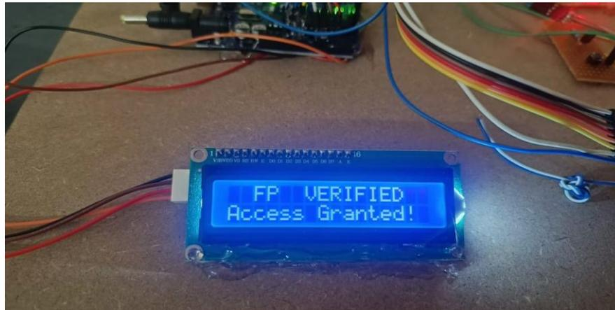
**Fig9 5.3 LCD Display**
