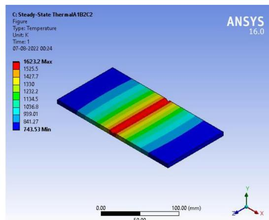
Fig-6.8 Temperature Distribution of A<sub>1</sub>B<sub>2</sub>C<sub>2</sub>
