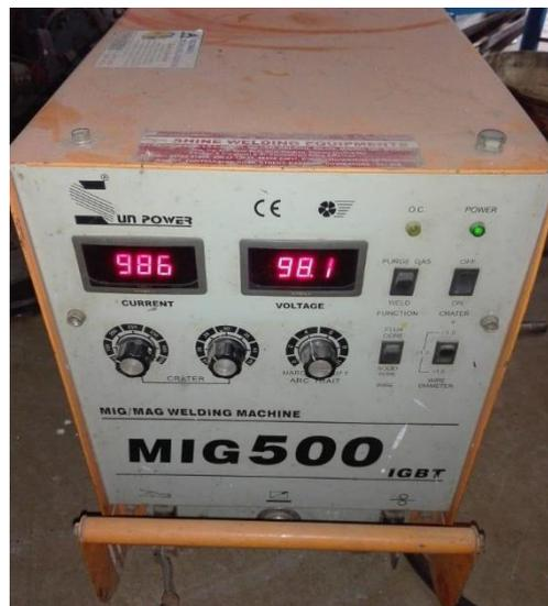
For this welding investigation the sun power MIG 500 IGBT machine was used with flux cored filler rod.
