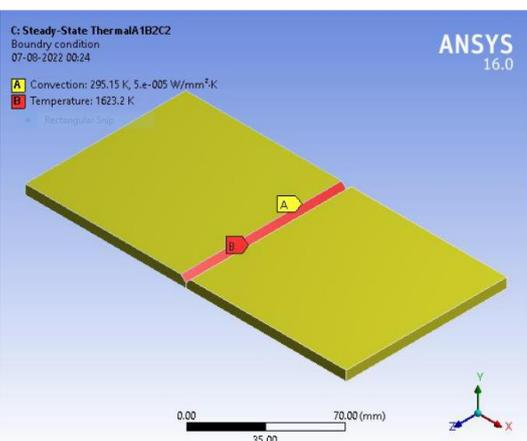
Fig-6.7 Boundary Condition of A<sub>1</sub>B<sub>2</sub>C<sub>2</sub>.
