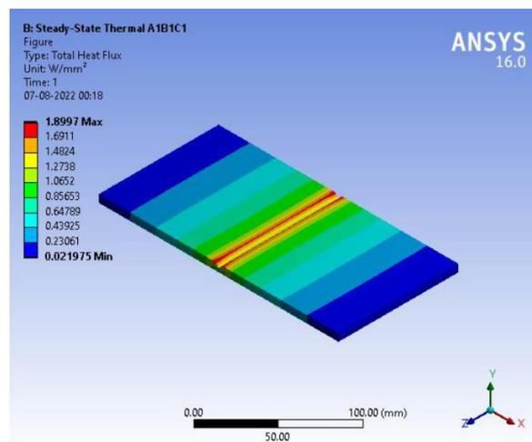
Fig-6.6 Directional Heat Flux of A<sub>1</sub>B<sub>1</sub>C<sub>1</sub>
