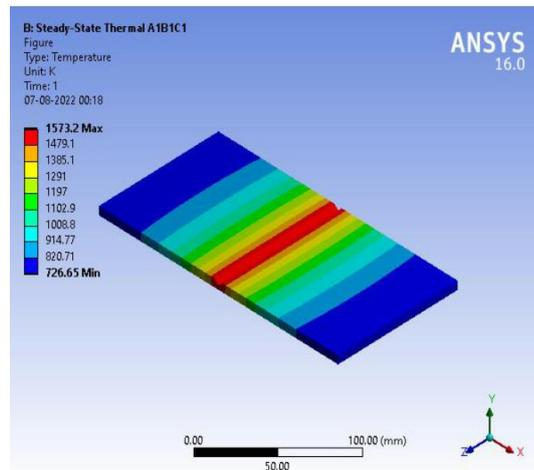
Fig-6.4 Temperature Distribution of A<sub>1</sub>B<sub>1</sub>C<sub>1</sub>
