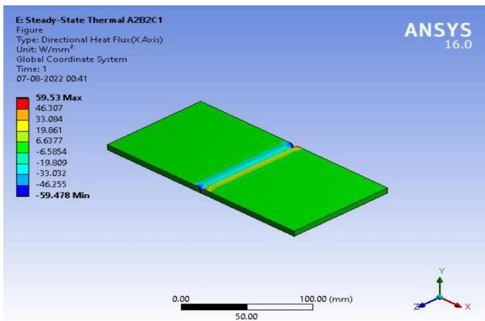
Fig-6.18 Directional Heat flux
