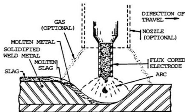
Figure1.1 Flux core Arc welding
