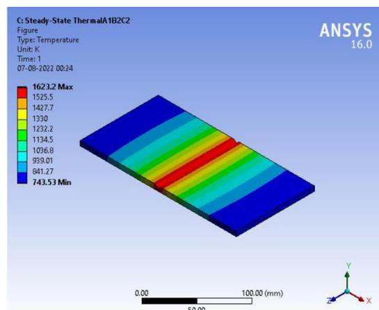
Fig-6.8 Temperature Distribution of A<sub>1</sub>B<sub>2</sub>C<sub>2</sub>
