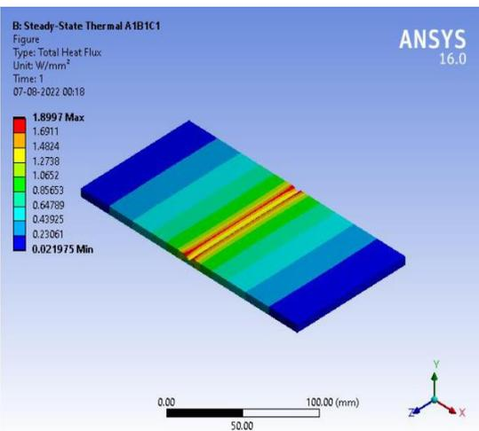
Fig-6.5 Total Heat Flux of A<sub>1</sub>B<sub>1</sub>C<sub>1</sub>.
