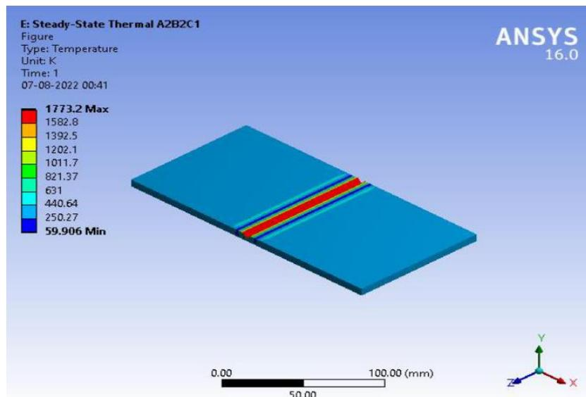
Fig-6.16 Temperature Distribution of  $A_2B_2C_1$
