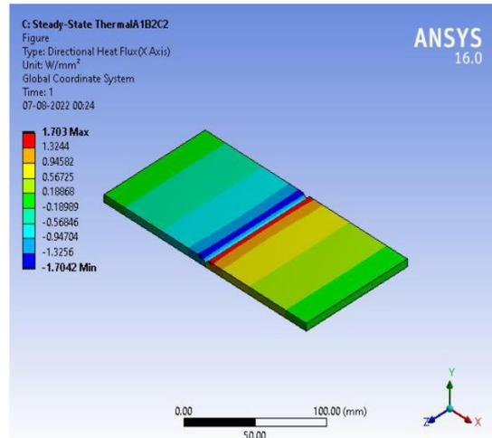
Fig-6.10 Directional Heat Flux of  $A_1B_2C_2$
