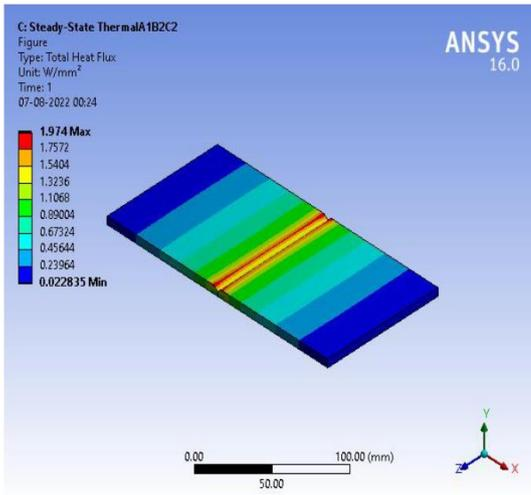
Fig-6.9 Total Heat Flux of  $A_1B_2C_2$
