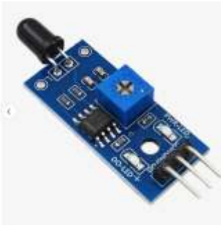
Fig -4: Flame Sensor
