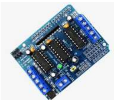
Fig -5: L293D Motor Driver
