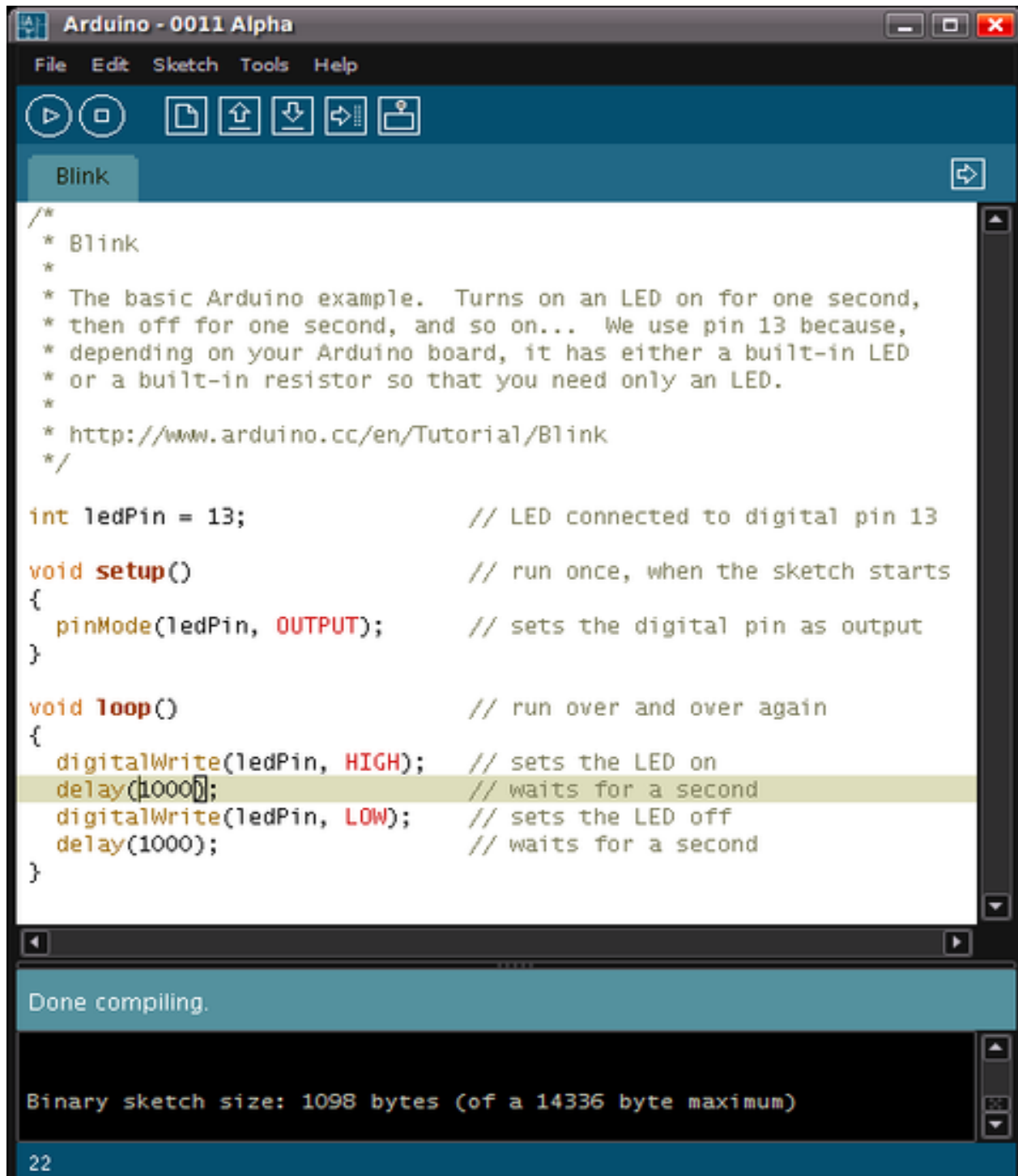
Figure 4 A screenshot of the Arduino IDE showing the "Blink" program, a simple beginner program
