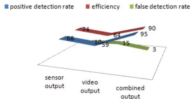
Figure 3. Comparison of sensor node, video node and combined outputs.
