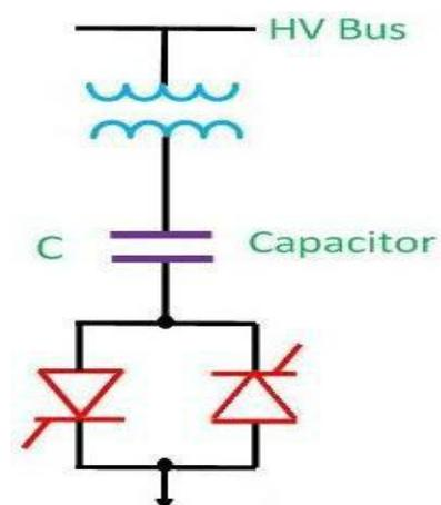
Fig.1 Thyristor Switched Capacitor (TSC)
