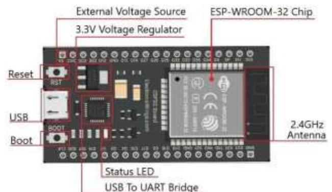
**Figure 2. ESP32 Microcontroller**
