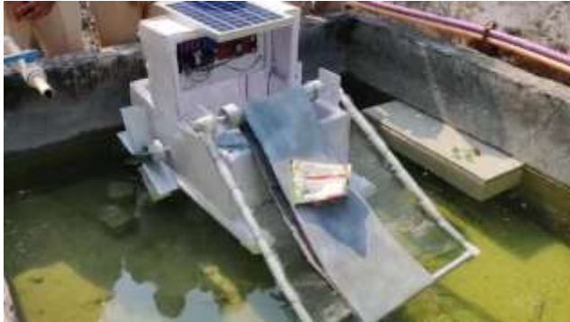
Fig. 7. Floating Debris Scooper Robot
