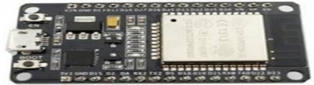
**Fig.2 ESP32 microcontroller**
