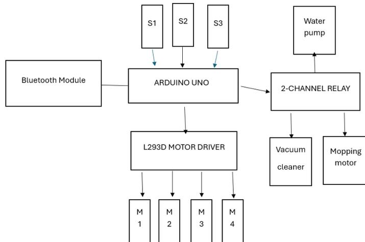
Fig- 4 Block Diagram of Floor Cleaning Robot
