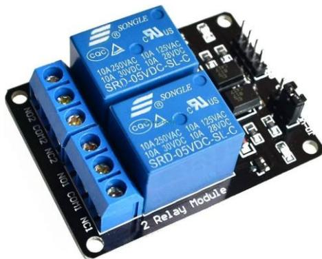
Fig2. Relay Module
