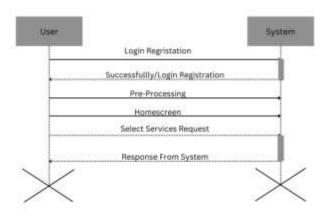
This diagram illustrates the chronological sequence of interactions between the 'User' and the 'System' for typical user operations. It begins with the login/registration process, followed by initial system pre-processing, display of the homescreen, and subsequent user requests for services and the system's corresponding responses
