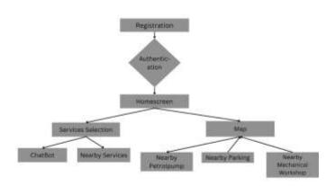
This diagram provides a high-level overview of the application's user navigation paths. It illustrates the primary routes a user can take after successful registration and authentication, branching from the main Homescreen to various core functionalities such as service selection (including chatbot support and nearby services) and map-based exploration (for petrol pumps, parking, and mechanical workshops)."
