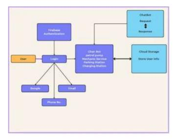
This diagram illustrates the high-level data flow within the application, starting from user authentication and extending to interactions with core service functionalities. It depicts how user login is handled via Firebase Authentication (supporting Google, Email, and Phone Number methods) and how central application services communicate with cloud storage and the chatbot component
