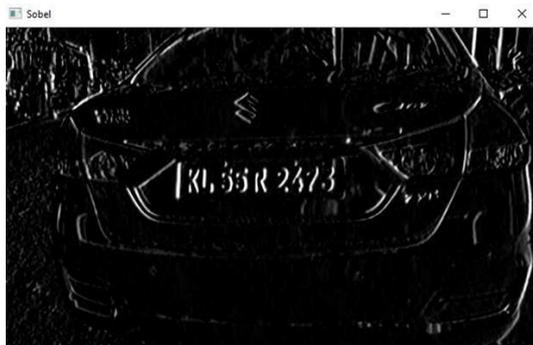
Figure 3.7: Imageprocessing using sobel technique
