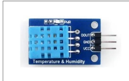
Fig- 3: DHT11 Temperature and Humidity Sensor
