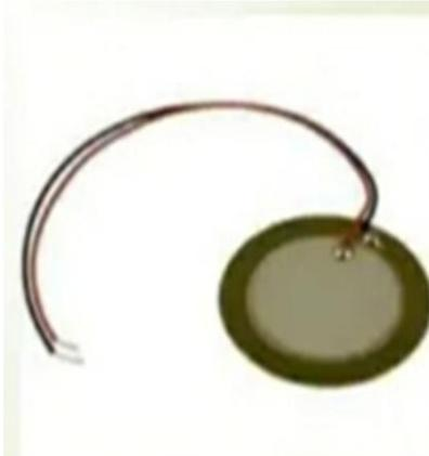
Fig 1. Piezoelectric Sensor
