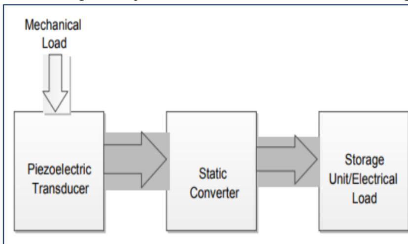
***Fig :3 Schematic diagram of a vibrating piezoelectric Harvester model***
