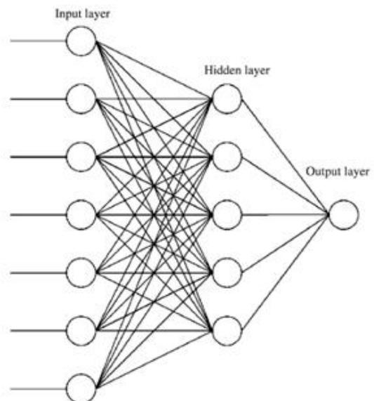
Fig. 4. illustrates the architecture of the typical three-layered feedback neural networks model.
