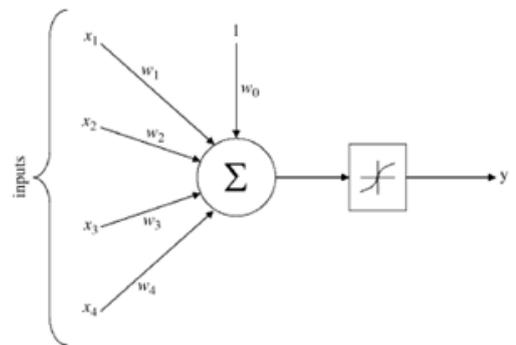
Fig.3. Internal structure of Neuron
