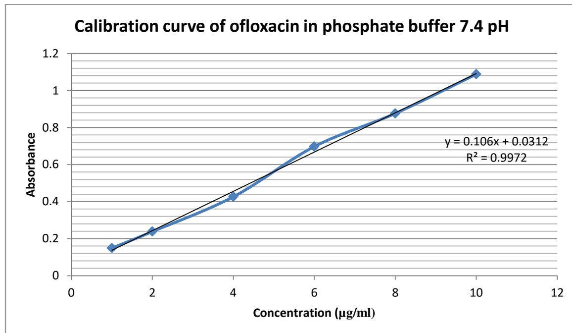
**Fig no. 2:** calibration curve of Ofloxacin in phosphate buffer
