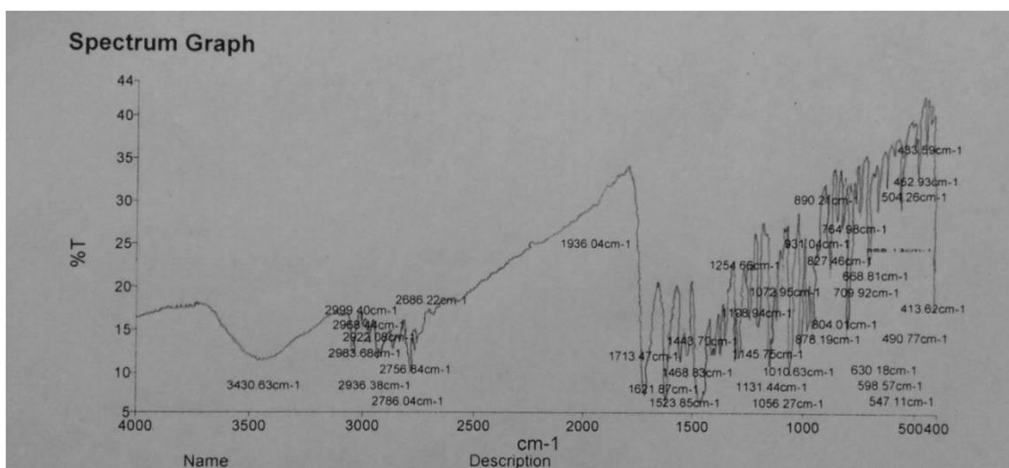
Figure no.5: FTIR spectra of pure drug and sodium alginate
