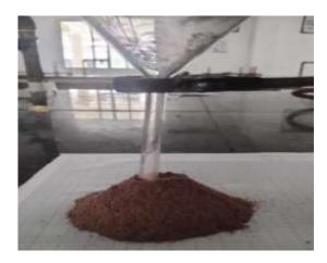
Fig. 9: Angle of Repose
