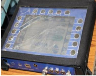
Fig. 3.2.1 FFT Analyzer
