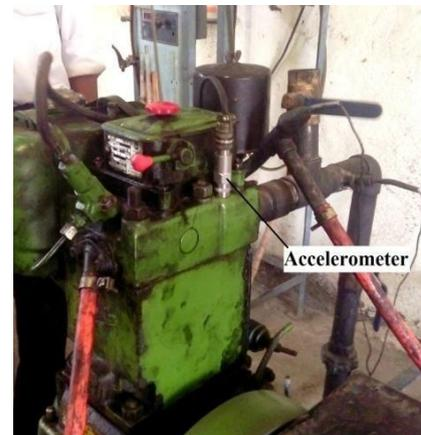
Fig. 3.2 Accelerometer mounted on Cylinder Head
