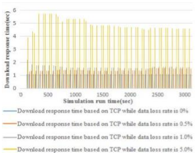
Fig14: Download response time based on TCP in the environment of different data loss rates
