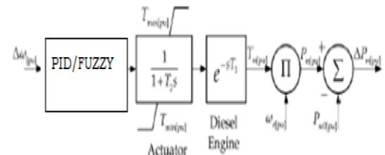
Fig. 2: Diesel motor model
