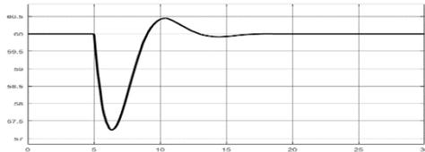
Fig 7 Frequency Response using Fuzzy Logic Controller
