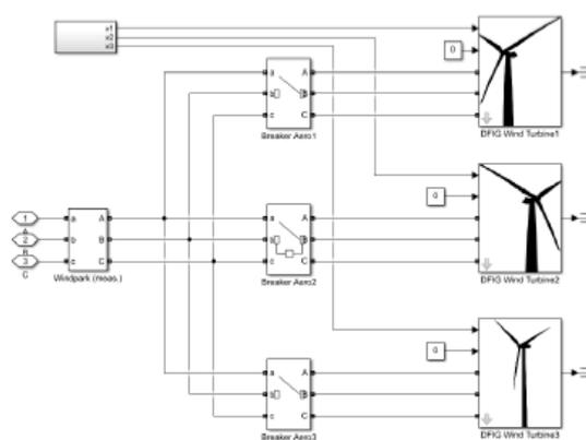
Fig. 3: Model of the wind farm subsystem
